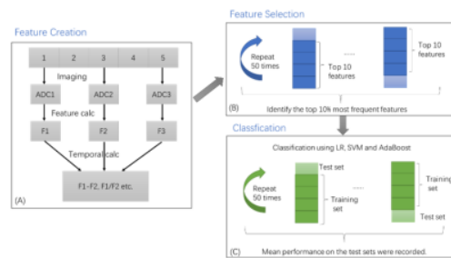
Figure 1. Illustration of feature creation, feature selection and classification process used in this study. Five-fold cross-validation with fifty repetitions was used in the feature selection part to select the most stable features, and used in the classification process to estimate the stability of the prediction.
